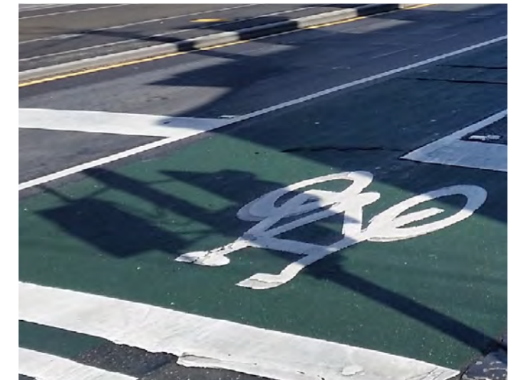
Bike boxes at signalised intersections allow cyclists to wait at the front of the line of waiting cars increasing visibility and safety.
