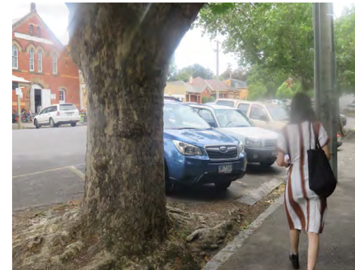
Remove some of the asphalt around the base of trees to increase the pervious surface
