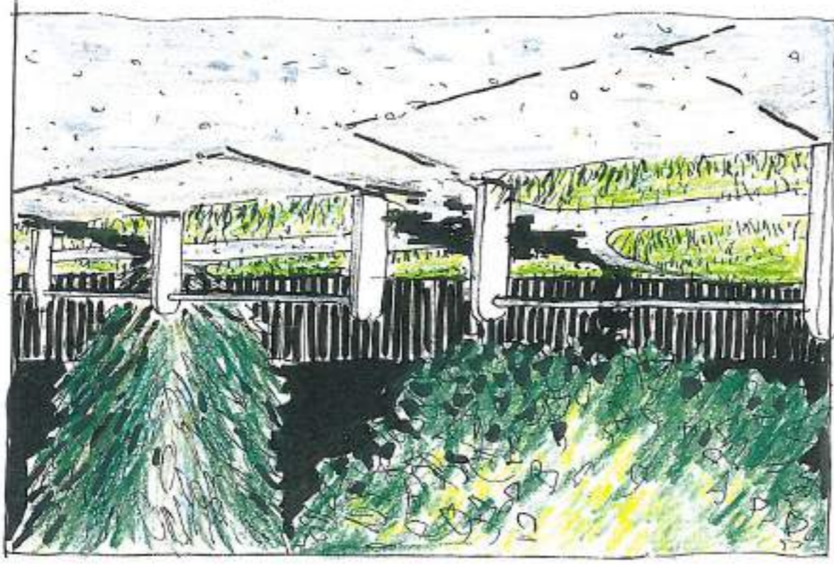
The sketch illustrates a less complicated treatment of the reserve boundary. The posts are off white painted hardwood and rail is galvanized pipe.
