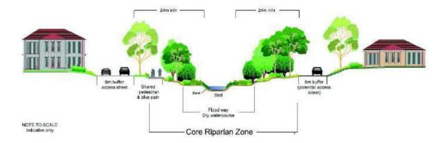
Figure 3: Typical Watercourse Cross section (Not to Scale)
