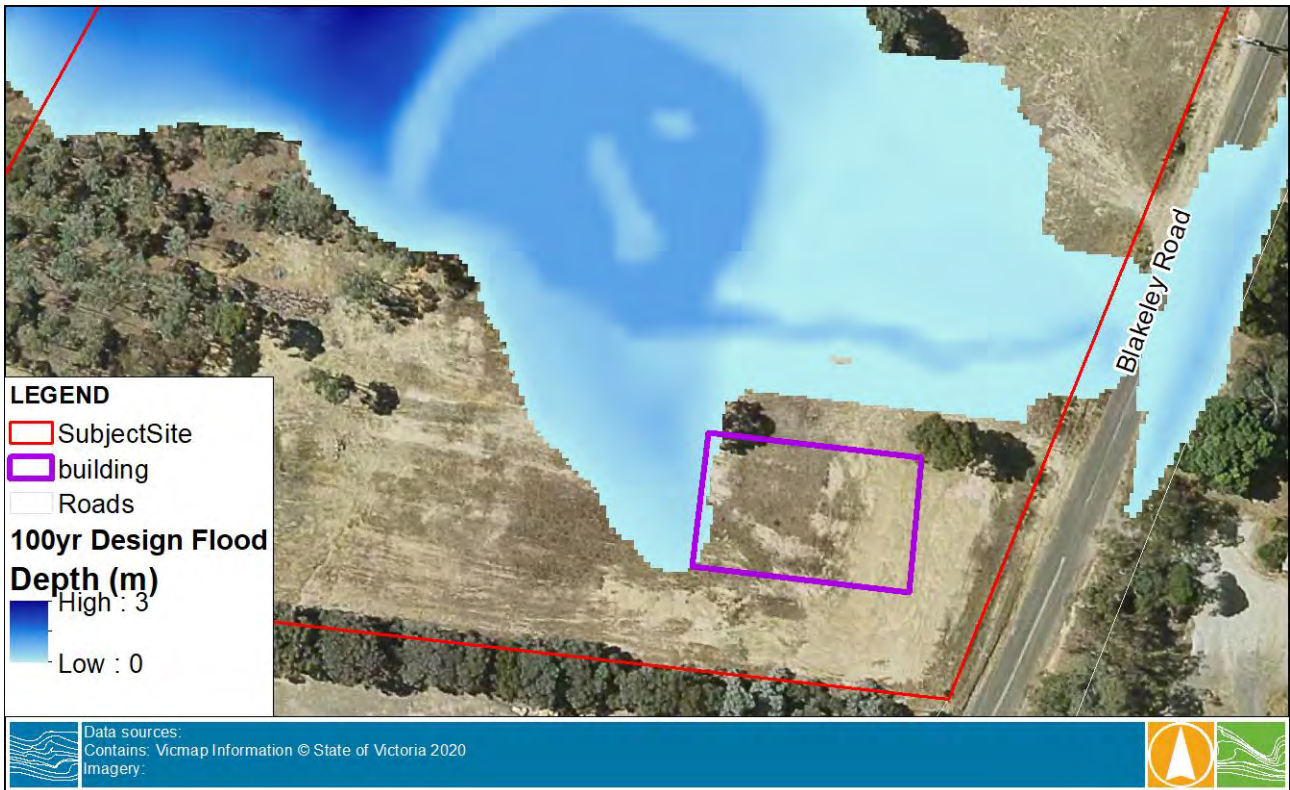
Figure 10-1 Indicative 1% AEP Flood Extent and Flood Depths
