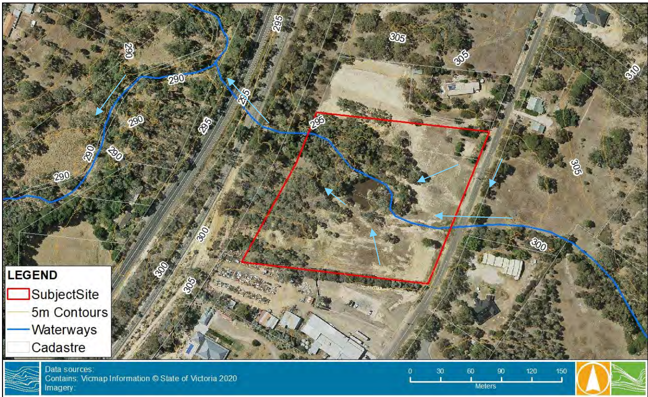
Figure 7-3 Drainage Flow Paths (indicated by arrows)
