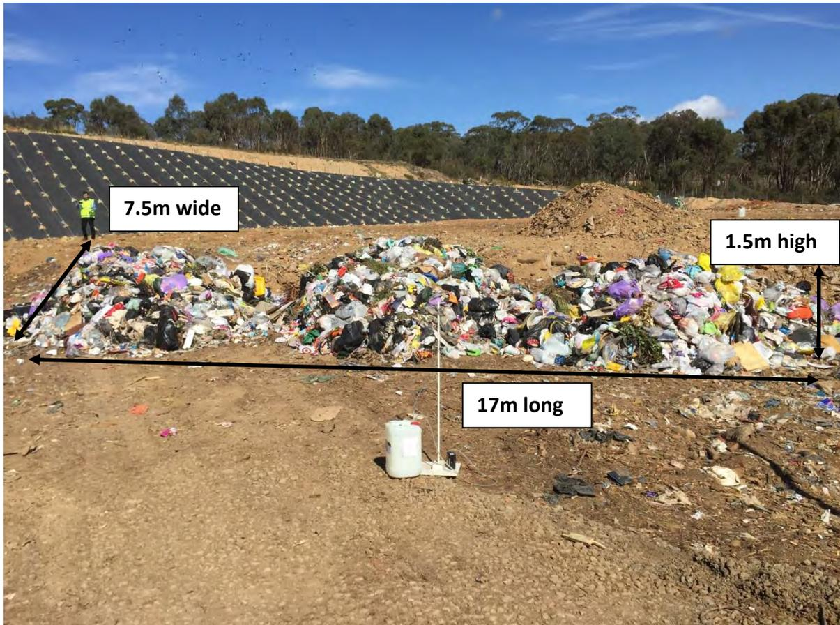
Test 3 was conducted at the active tipping face immediately after the received material was compressed and covered with temporary cover (clean fill). The following photographs show the process part way to completion.
