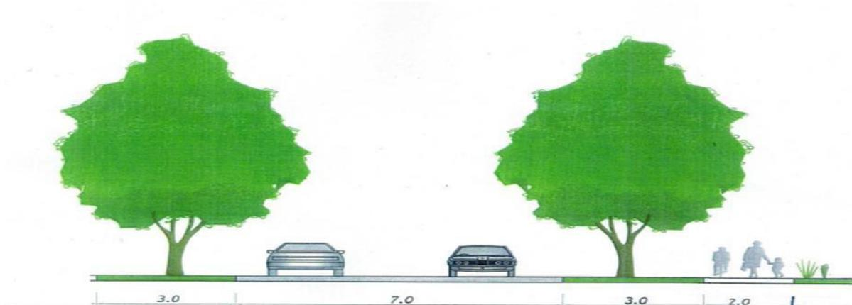
Figure 4: Typical Collector Road Cross Section (Source: Beveridge Williams; Not to scale)
