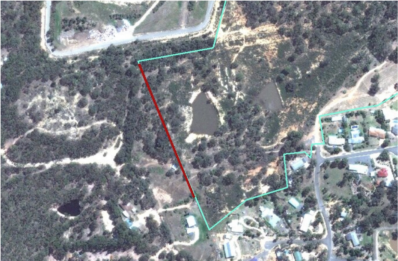
Plate 11 - The area that is currently unfenced is marked in red. This boundary is proposed to be fenced using a post and wire design with 1-2 strands of wire.
