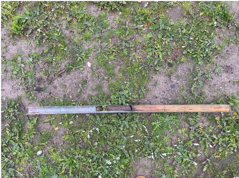
6. Soil Sampling BH02 to 1.20mBGL compaction of direct push tube
